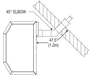
Horizontal Venting Maximum 47.5" (1.2 m) with 45° elbow. 45° elbow can be purchased from a local hardware store.
